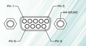
\* Connection to +15V OPEN, Connection to -15V: CLOSE (Normally closed valve model) Connection to +15V CLOSE, Connection to -15V: OPEN (Normally open valve model)
